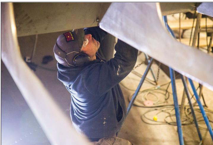
Leigh O'Conner works on the extension of the Kariel's stern, which will help to increase flotation to improve the boat's safety and efficiency.
