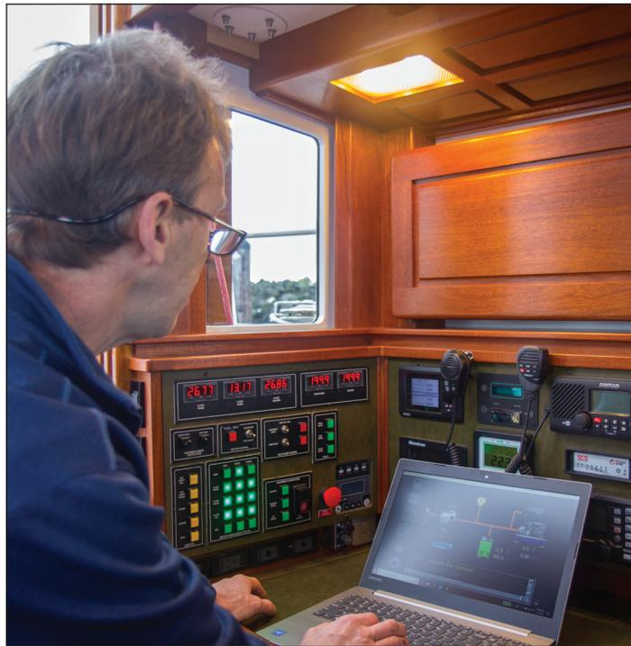
Chris Sanok demonstrates how the boat's batteries and systems are monitored by a computer, which can also be transmitted via Wi-Fi onto the boat owner's phone.
