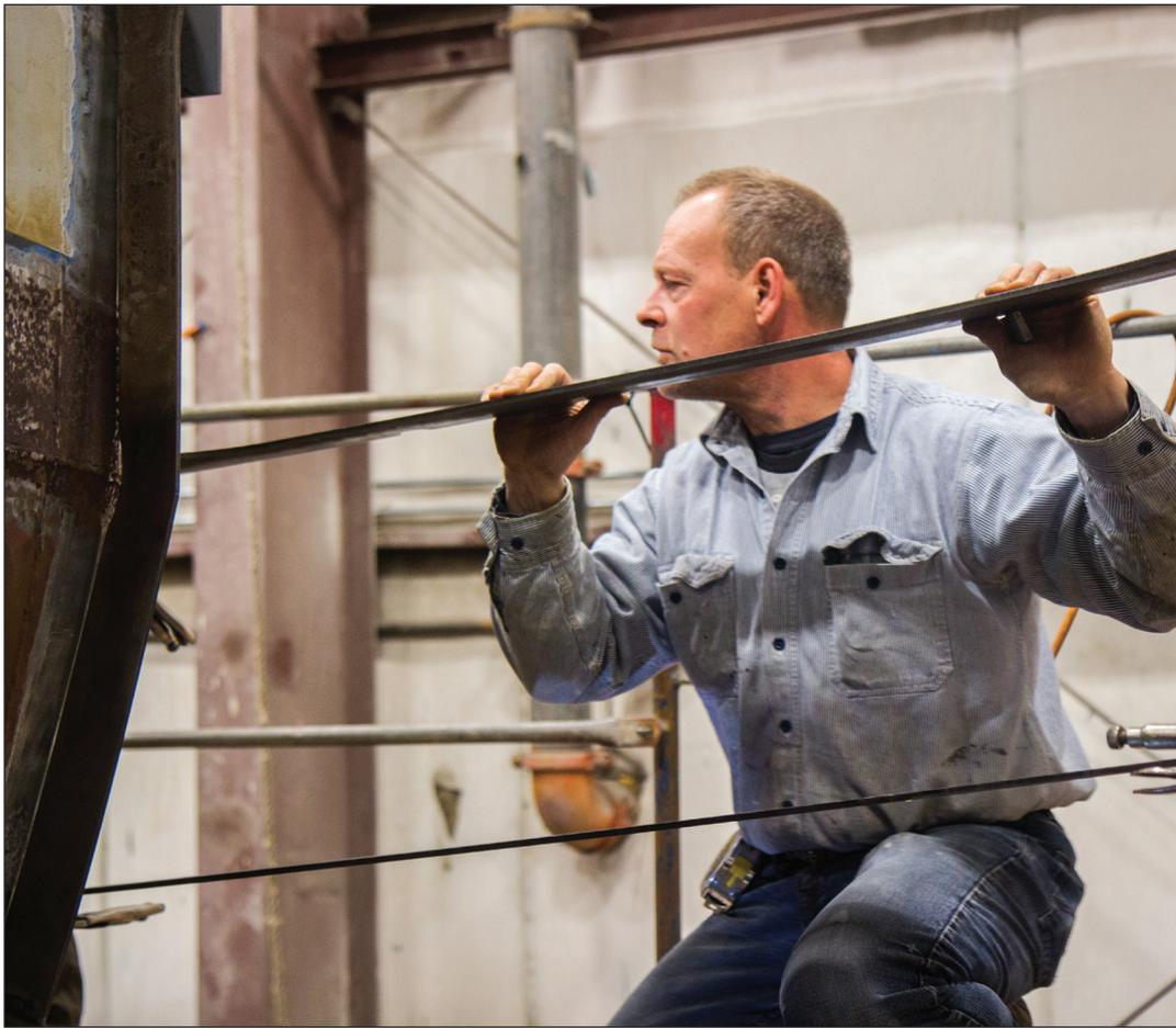
Shipwrights Brad Lato and Tim Hoffman work with steel parts cut by a computer to construct an extension to the stern of the commercial fishing boat Kariel.
